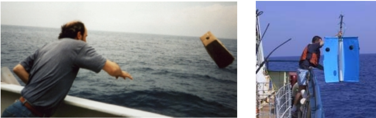
Figure 6. Two possible ways of deploying a CODE drifter: closed in its cardboard box for protection (left) generally if it is thrown from a moving vessel or after it has been removed from it (right).
