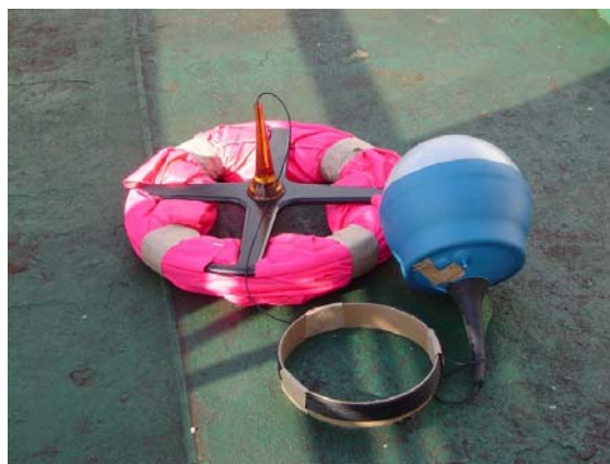
Figure 4. Before deployment paper tape binds the SVP drogue and tether. The latter can be wrapped around a cardboard ring to avoid kinking. The upper portion of the tether attached to the surface
