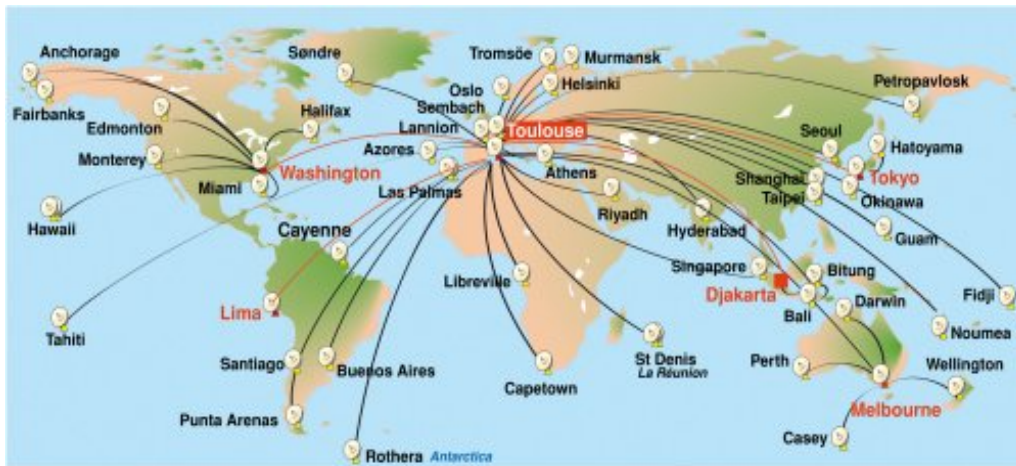
Figure 9. Position of the stations that form the real time L-band antenna-network. Each of these receive real time data from the satellites and retransmit them to processing centers. Two of the main receiving stations are in the USA (Wallops Island and Fairbanks) one in Norway (Svalbard).
