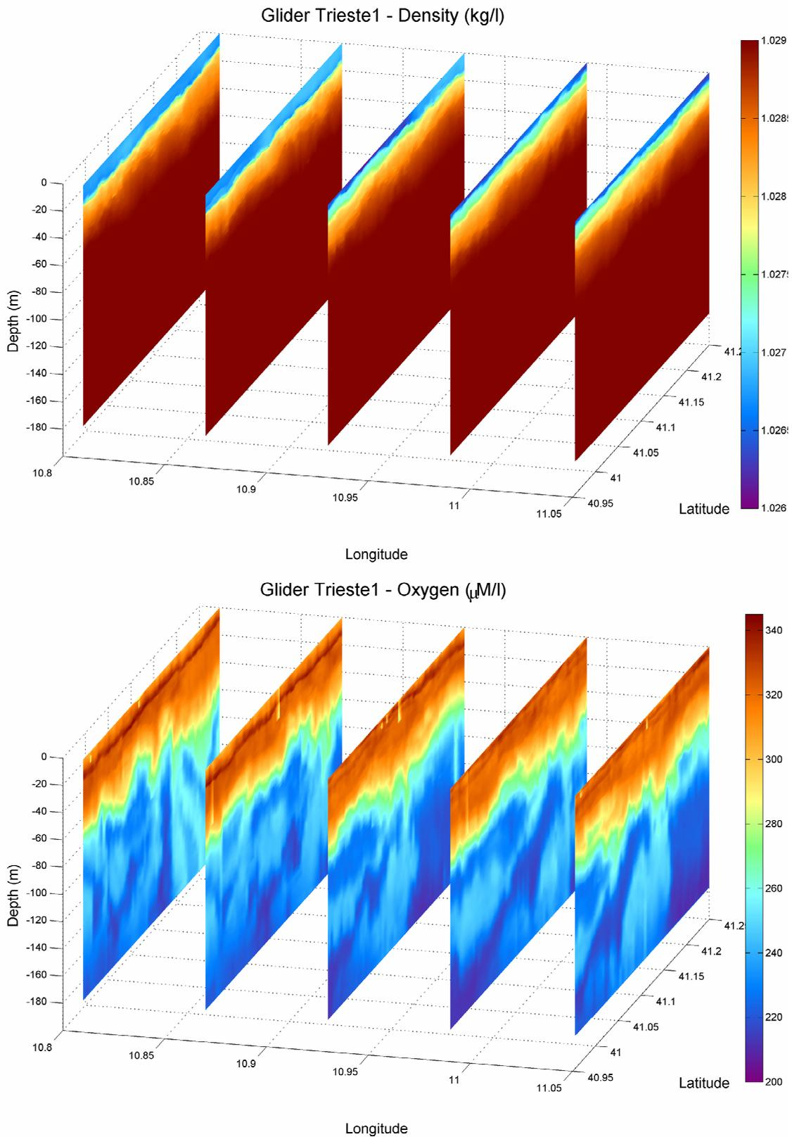
**Fig. 15** Color-coded contours of density and oxygen ( $\mu\text{M/l}$ ) along the drifter track between 4 and 180 m.
