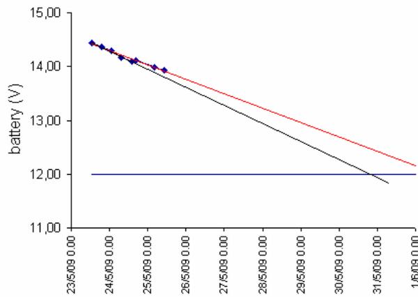
**Fig. 9** Monitoring of the battery voltage. Estimate computed from the initial consumption (black line) and estimate after 3 days (red line). The blue line of 12 V indicate the abort mission limit.
