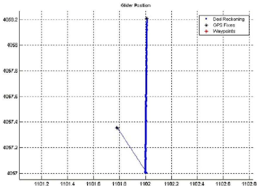
**Fig. 7** Analysis of the glider position after the deployment (northern asterisk). Even if we do not received any communications from the glider, it sailed southward reaching the initial waypoint. The glider drifted a bit northwestward when at surface.
