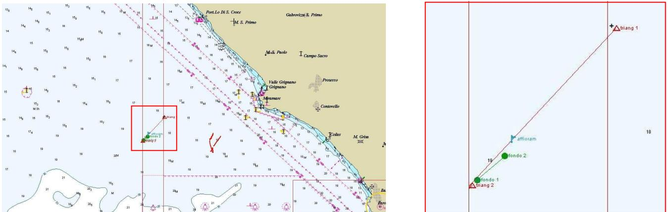
**Fig. 4** Left: the test mission area in the Gulf of Trieste. Right: waypoints of the first mission (from north to south, red triangles), surfacing point (light blue flag) and waypoints of the second mission (from south to north, green dots).
