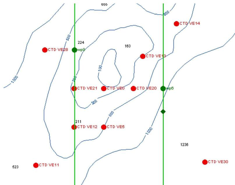
**Fig. 5** Close up of the optimized glider mission: glider track (green lines; northward on the left side and southward on the right), safety waypoints (green dots), surfacings (green diamonds) and CTD stations (red dots). The bathymetry is depicted with light blue isobaths.
