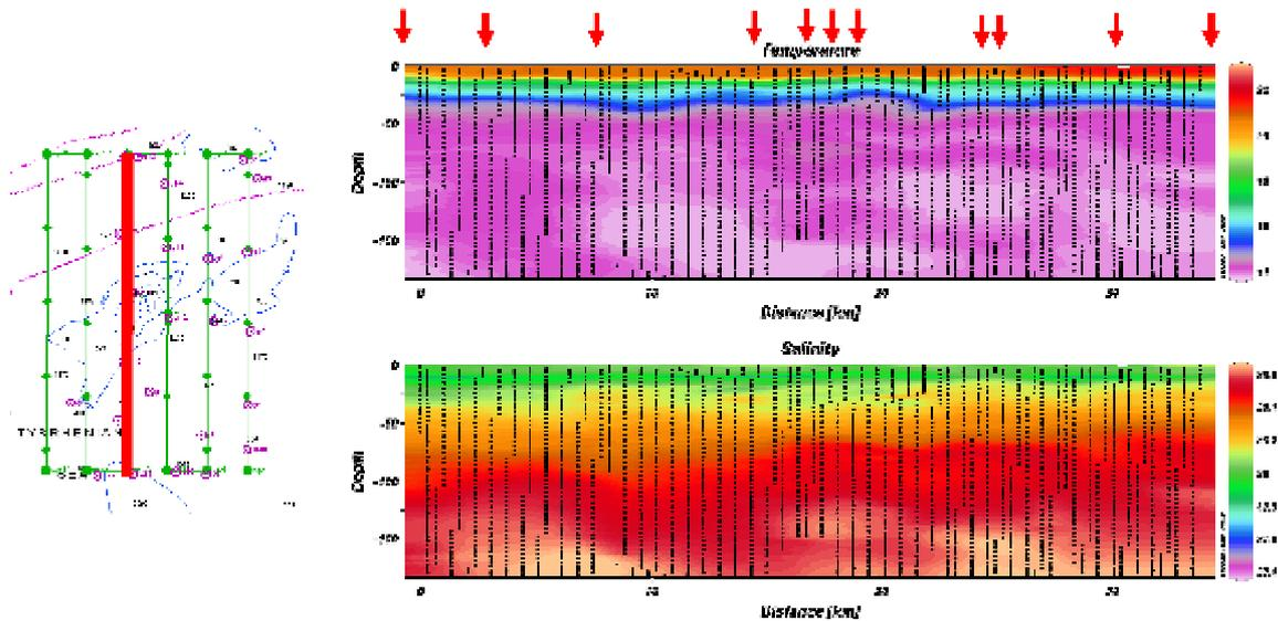
**Fig. 10** First data plots of the SBD files sent by the glider to the ogadock: transect location (on the left) and temperature and salinity contour plots (on the right). The red arrows on the upper part of the temperature plot indicate the CTD stations performed by the ship. Black dots indicate the actual data points. Temperature is in °C.
