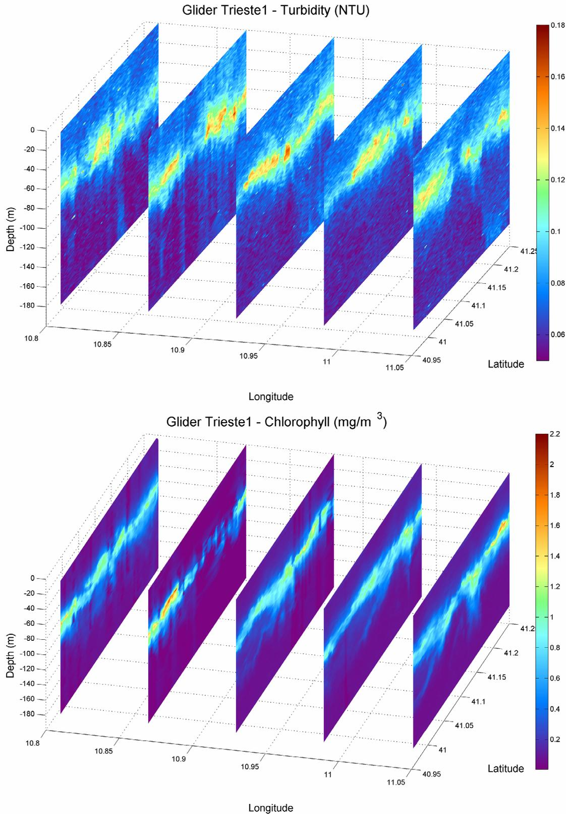
**Fig. 16** Color-coded contours of Turbidity (NTU) and Chlorophyll ( $\text{mg}/\text{m}^3$ ) along the drifter track between 4 and 180 m.
