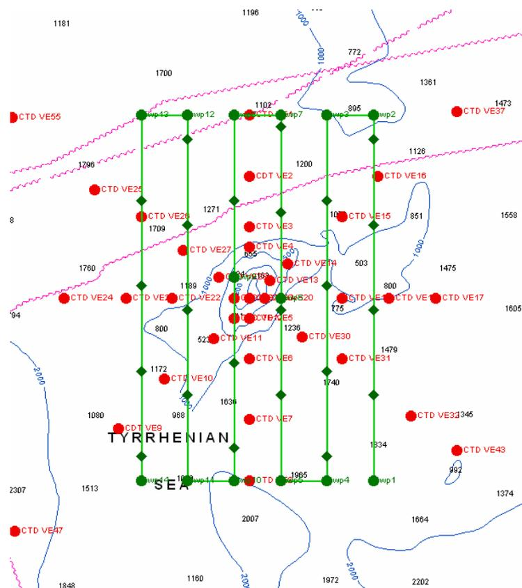
**Fig. 3** The optimized Tyrrmount09 glider sampling scheme: glider track (green lines from the southeastern corner to the southwestern one), waypoints (green dots), surfacings (green diamonds) and CTD stations (red dots). The bathymetry is depicted with light blue isobaths.
