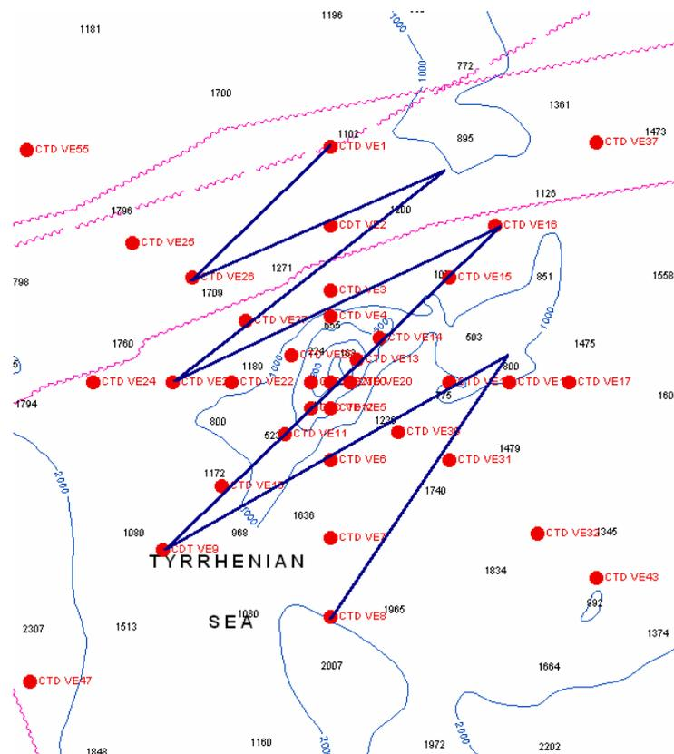
**Fig. 2** The initial sampling scheme proposed by CNR: glider track (dark blue lines from north to south) and CTD stations (red dots). The bathymetry is depicted with light blue isobaths.
