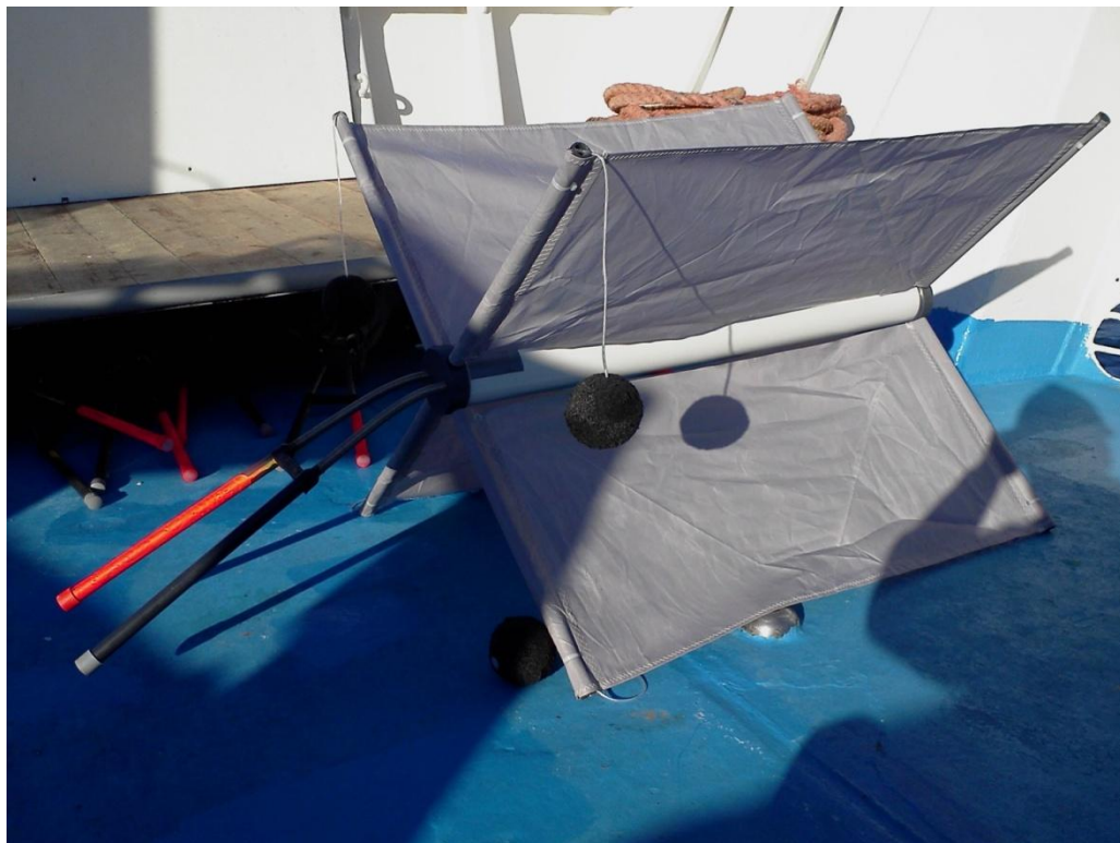
Figure 3. Drifter ready to be deployed. One of the antennas has been painted in orange to facilitate the recovery.
