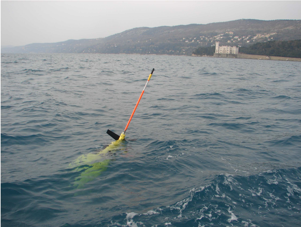
Fig. 1. The SeaGlider at surface in the Gulf of Trieste with the Miramare castle in the background.
