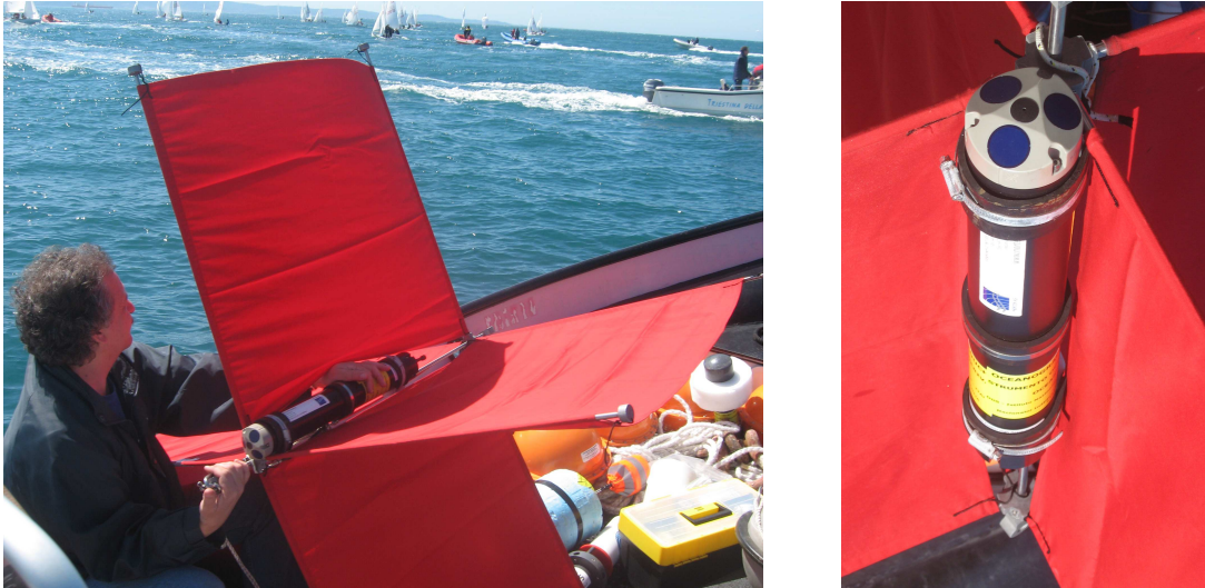
Fig. 12. CODE drifter with upward-looking ADCP from UAEGEAN
