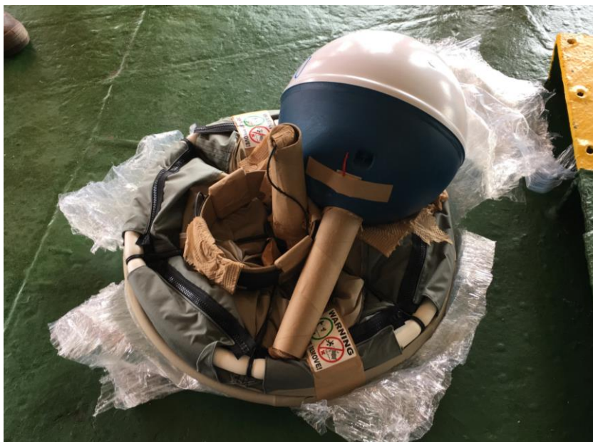
Figure 11. SVP drifter manufactured by Pacific Gyre on the deck of R/V Italica before deployment in the Southern Ocean in January 2016.
