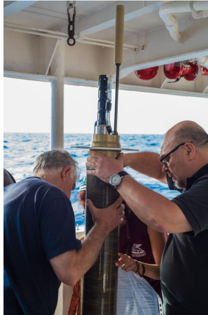
Figure 3. Deep Arvor float (WMO 6903200) before deployment on the R/V Aegea on 8 June 2016.
