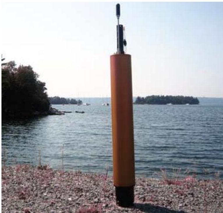
Figure 1. Photograph of a Nova float, with the CTD sensors and Iridium antenna at the top and blader (to change buoyancy) at the bottom.
