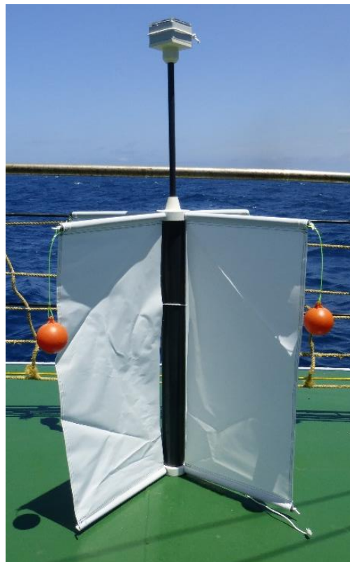
Fig. 4. CODE drifter (antenna, vanes and orange balls).
