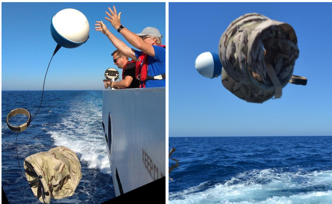
Fig. 12. Deployment of SVP drifters from R/V ALLIANCE (left) and R/V SOCIB (right).
