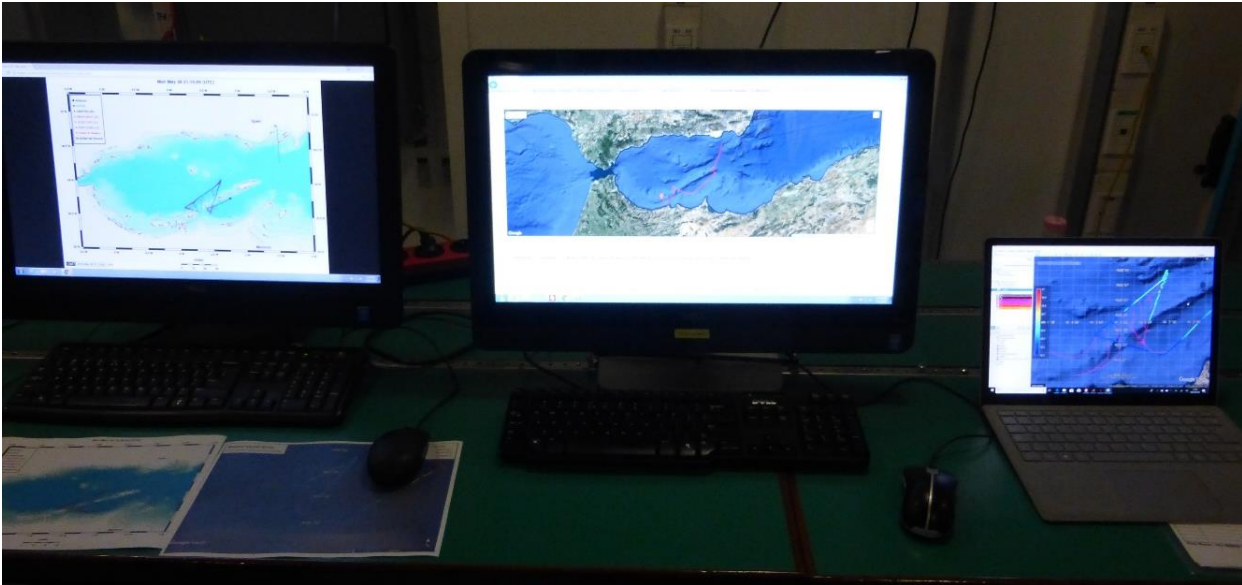
Fig. 13. Graphical displays of the drifter data used on R/V ALLIANCE for planning the drifter deployment and viewing their trajectories in real time.
