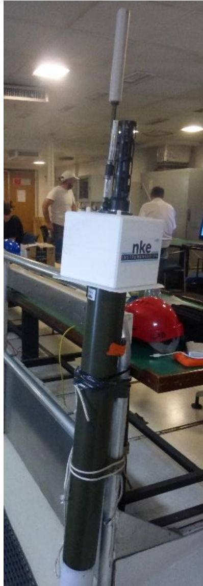
Fig. 6. Arvor float (with from top to bottom: Iridium antenna, CTD and bladder).
