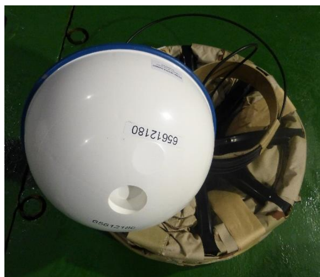
Fig. 1. SVP drifter (surface buoy and folded holey sock drogue).
