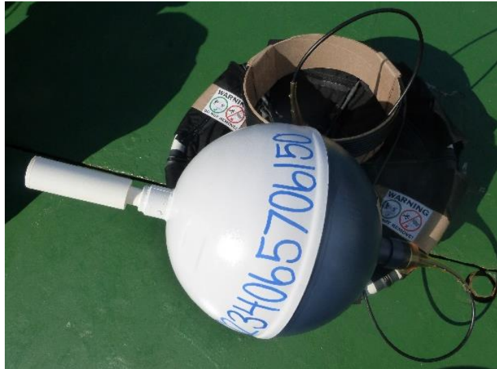
Fig. 2. SVPB drifter (surface buoy with barometer and folded holey sock drogue).
