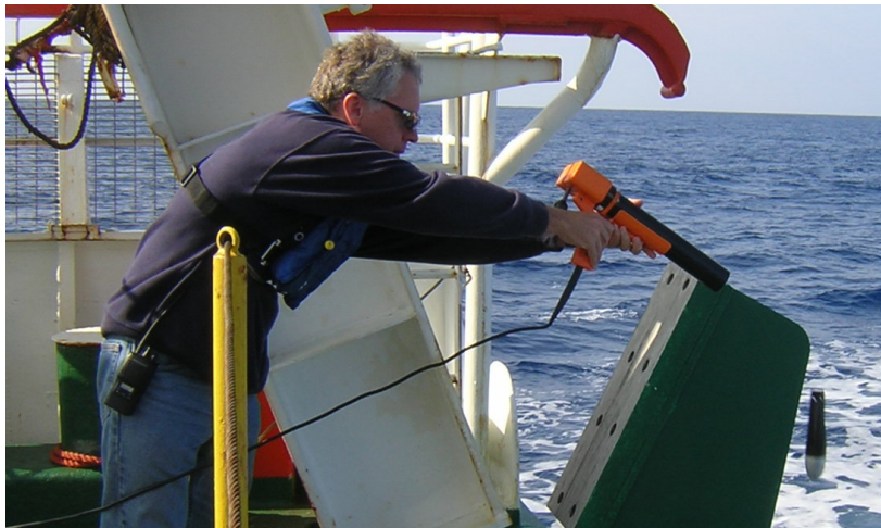
Figure 7. Picture of the launch of an XBT probe. The hand-held launcher and the probe are clearly seen.
