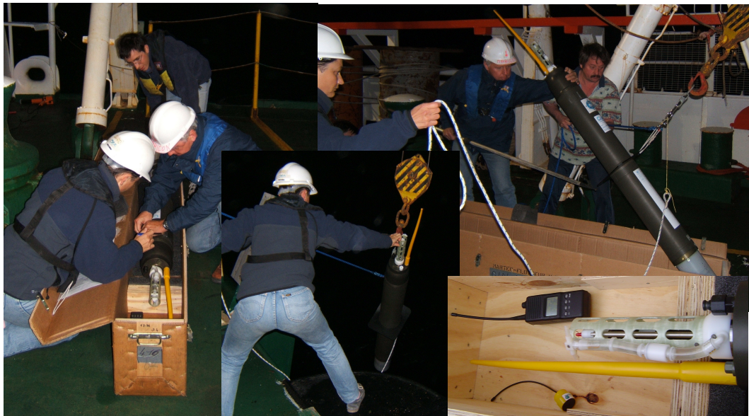
Figure 10. Pictures showing the deployment operations of a PROVOR profiler. Left: turning on the float. Bottom right: checking the float transmission (beeper, Telonics receiver, float antenna and CTD sensors). Center and top right: deploying the profiler using the A-frame.
