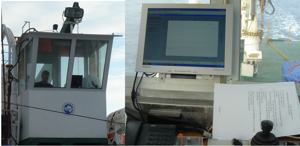
Figure 6. Pictures of the “caponera” where the Sippican MK21 USB acquisition system and computer were installed. Left: view of the “caponera” from the aft deck; right: inside the “caponera” with monitor showing the XBT acquisition graphics and the view on the ship’s stern.
