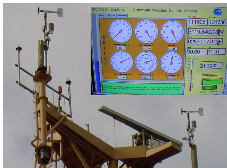
Figure 4. Picture of the two Meteorological stations mounted on R/V OGS-EXPLORA. Insert: real-time display of the meteorological observations as it appears in the laboratory.
