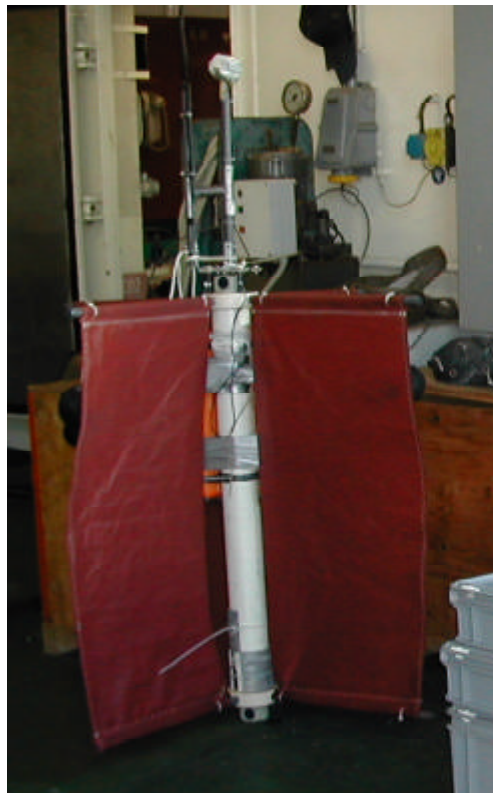
Figure 6. Prototype CODE drifter with two Nortek Aquadopp velocimeters, and the GPS and Argos antennas.
