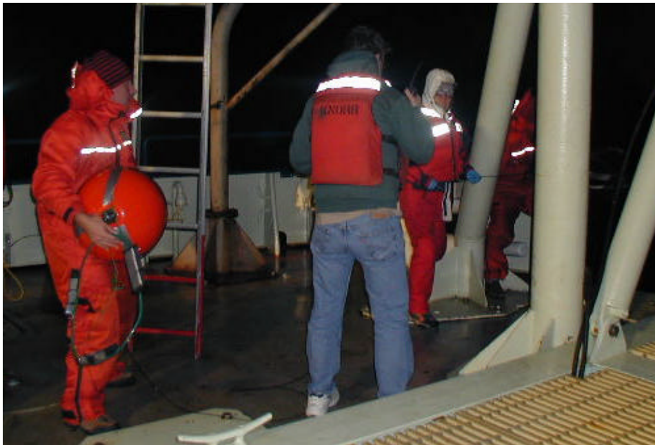
Figure 8. Deploying an optical drifter ( SVP/OCM) from the stern.
