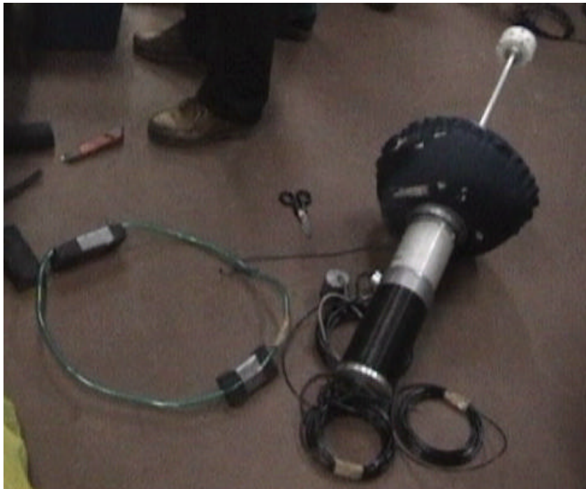
Figure 5. CMOD (XAN-3) drifter with thermistor chain.
