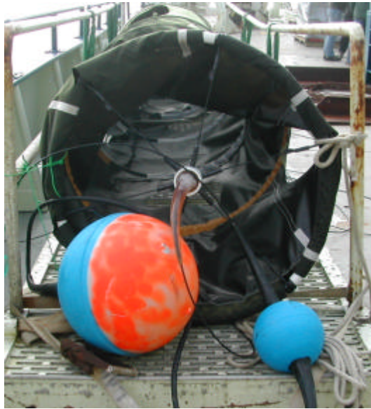
Figure 2. SVP drifter with holey-sock drogue, intermediate float (lower right) and surface ball (left).
