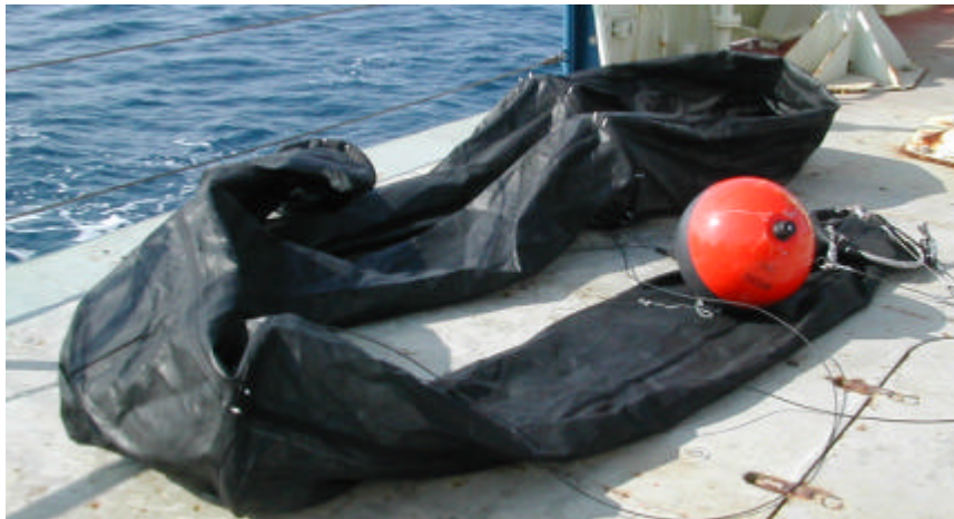
Figure 3. SVP/OCM drifter with sock drogue. The irradiance meter can be seen on the top of the red surface ball.
