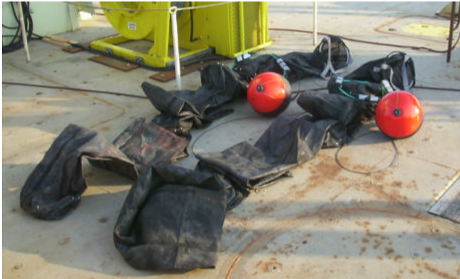
Figure 3. SVP/OCM drifters with sock drogues. The irradiance meters can be seen on the top of the red surface balls.
