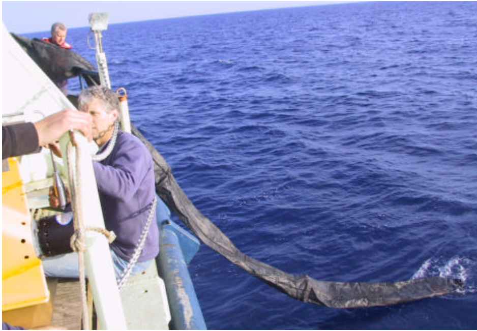
Figure 8. Deploying an optical drifter ( SVP/OCM) from the stern. The drogue is being paid out before tossing the surface ball.
