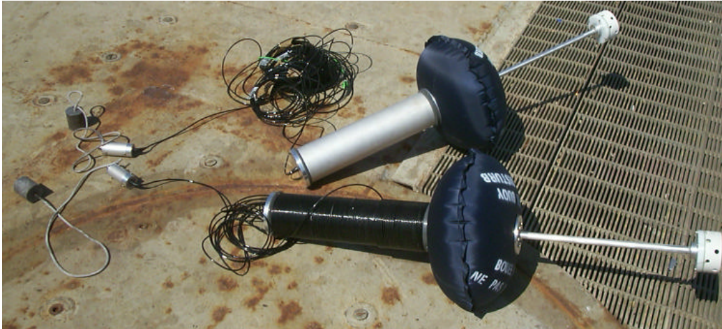
Figure 5. CMOD (XAN-3) drifters with thermistor chains.
