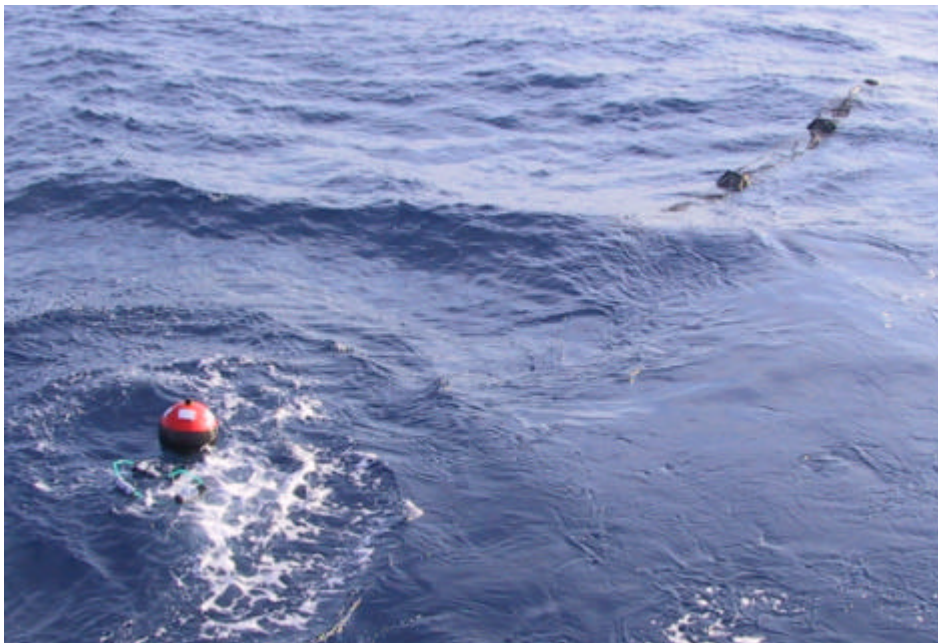
Figure 9. An SVP/OCM drifter just after deployment. The surface ball (bottom left) and drogue (before sinking, top right) are clearly seen.
