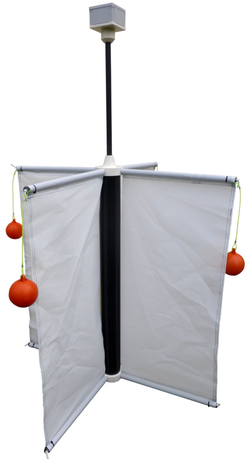
Figure 1. Low-cost CODE drifter equipped with LoRa transceiver in the box
