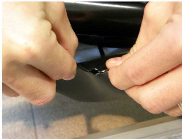
Fig. 6: The leak in the air bladder.
