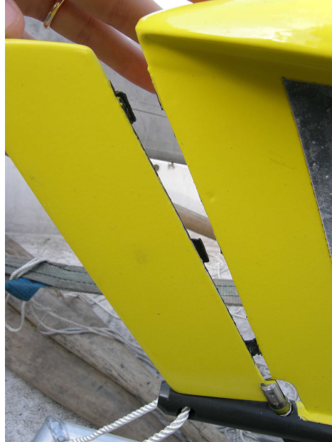
Fig. 4: The damage occurred on the rudder during the first leg.
