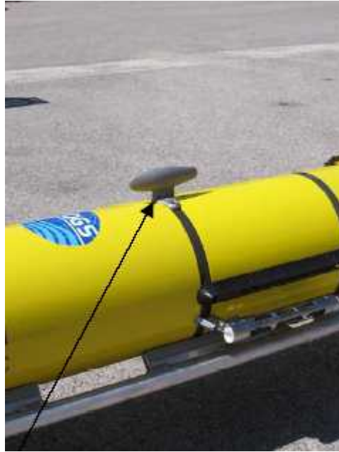
Fig. 3: The hook mounted on top of the mid hull section of the glider.
