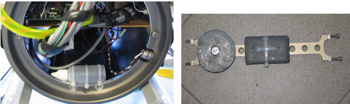
Fig. 2: Redistribution of the internal weights of the glider: bottle filled by plumb bobs (left) and load rail (right).
