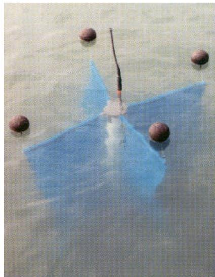
Figure1: Modified CODE drifter floating in the water.
