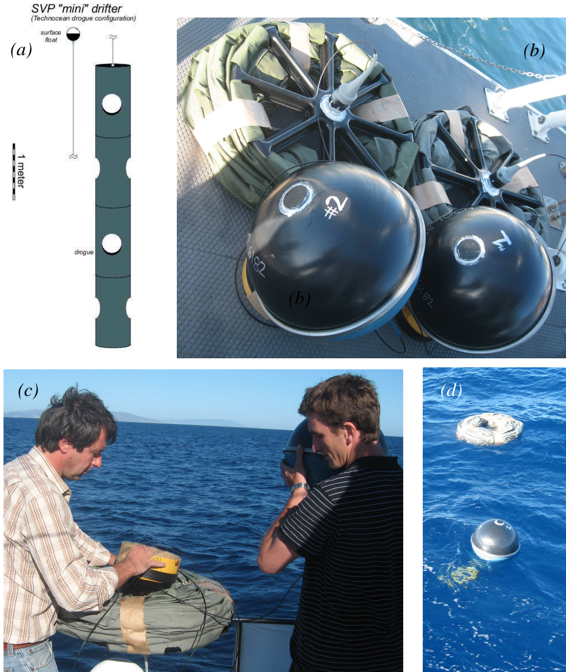
Figure 2. (a) Schematic diagram of the SVP “mini” drifter. (b) Two SVP drifters ready to be deployed on the ship’s deck. (c) Deployments of a SVP drifter during MILONGA. (d) SVP drifter just deployed at sea.
