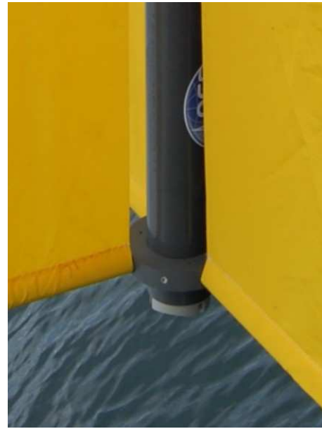
Fig. 3. The Aquadopp current profiler at the bottom of the prototype drifter.
