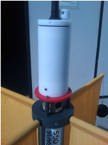
Fig. 2. The GPS/GSM position/transmission module and the Aquadopp current meter head visible below the red PVC plate.
