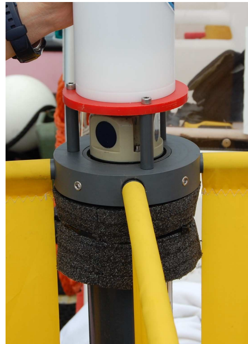
Fig. 11. The floating ring added around the tube below the top current meter to correct buoyancy.
