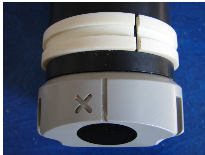
Fig. 9. The collar mounted on the Aquadopp profiler in correspondence of the indentation (see also Fig. 8).
