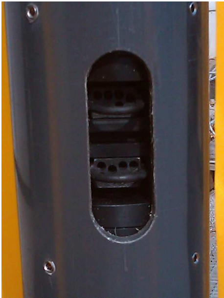
Fig. 5. The two end bells of the two Aquadopps mounted on the drifter.
