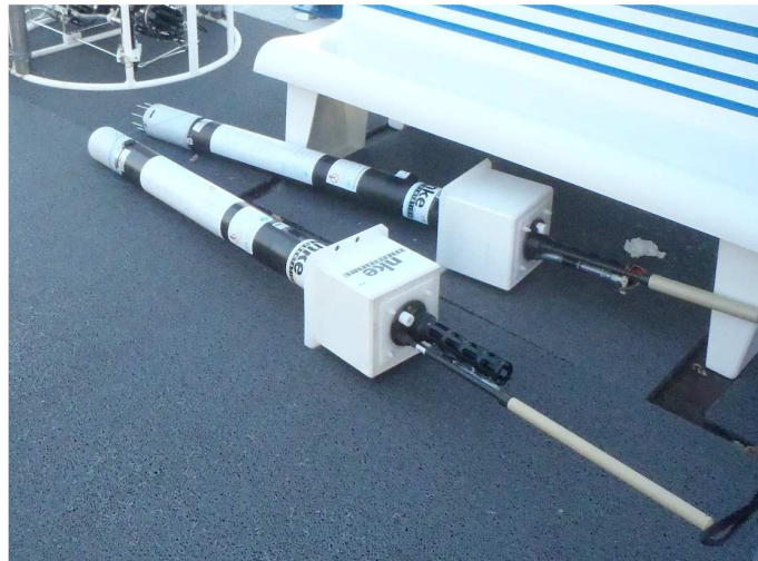
Figure 5. Argo floats lying on the aft deck of R/V SOCIB before deployment.
