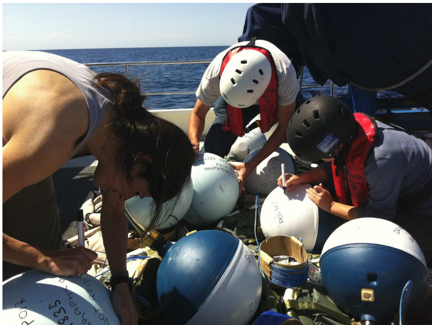
Figure 2. Preparation of SVP drifters (labelling and switching on) prior to deployment on R/V SOCIB.
