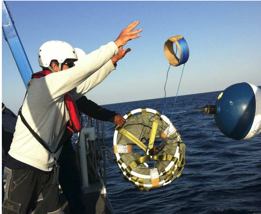
Figure 3. Deployment of a SVP drifter in the eastern Alboran Sea. The surface buoy, tether and hoely sock drogued (folded) are clearly visible.
