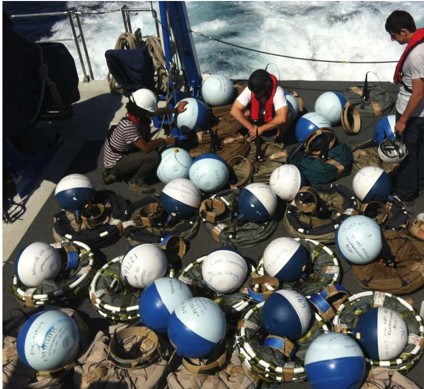
Figure 1. SVP drifters lying on the aft deck of R/V SOCIB before deployment.
