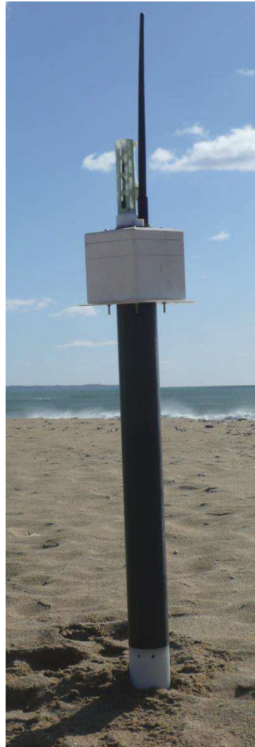
Figure 2. Photograph of an ARVOR-L float, with the CTD sensors and Argos antenna at the top and blader (to change buoyancy) at the bottom.
