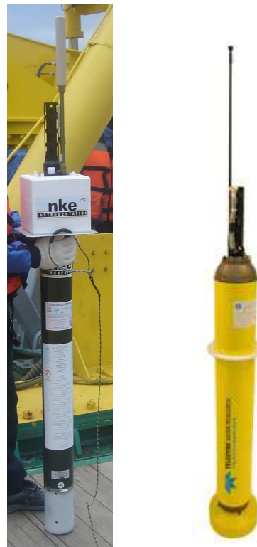
Figure 2. Arvor (left) and Apex (right) floats, with the CTD sensors and Argos Iridium/antenna at the top and bladder (to change buoyancy) at the bottom.
