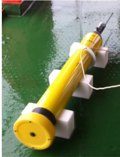
*Figure 4. Apex float (WMO 6901821) ready to be deployed in the Southern Ocean (Pacific Sector) on the deck of R/V Italice.*
