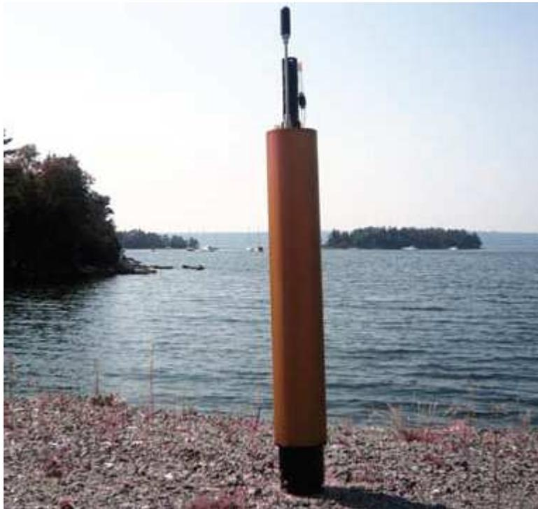
*Figure 1. Photograph of a NOVA, with the CTD sensors and Iridium antenna at the top and bladder (to change buoyancy) at the bottom.*
