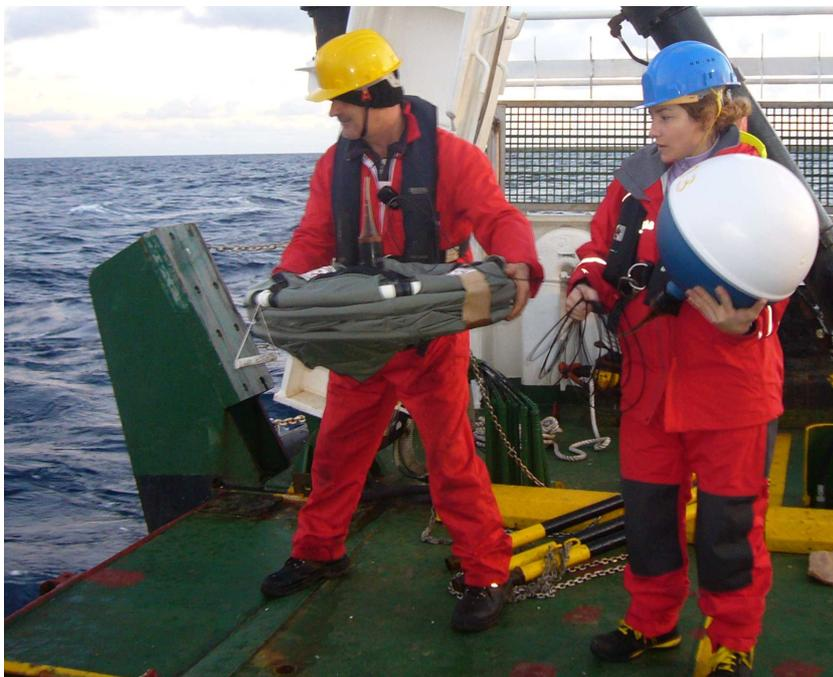
*Figure 14. Deployment of an SVP drifter during the ADREX campaign from R/V OGS Explora in the northern Ionian Sea in February 2014.*
