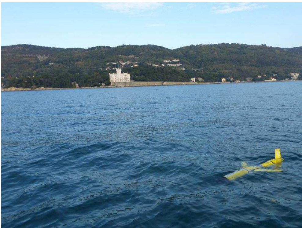
Figure 18. Photograph of the Slocum glider “unit 403” with the new 1000-m forward section being tested in the Gulf of Trieste on 27 October 2015.
