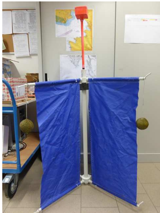
Figure 17. The low-cost CODE drifter manufactured at OGS.
