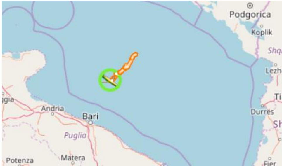
Figure 20. Glider “unit 403” trajectory during the CONVEX17 experiment (concluded prematurely) in the South Adriatic Sea. The glider symbol indicates the last position of the instrument. Orange symbols correspond to surfacing locations.
