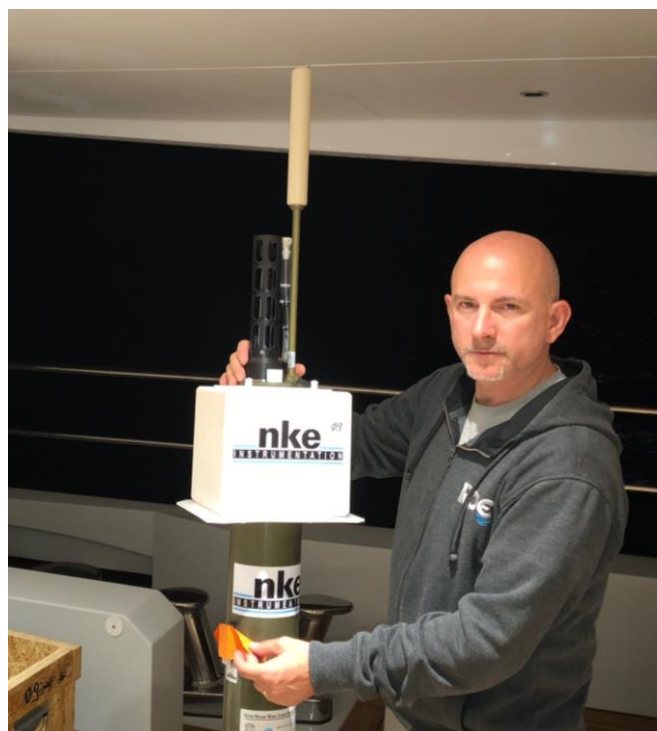
Figure 2. Captain L. Triggiani removing the magnet from an Arvor float on M/Y ROE before deployment of the float in the Ionian Sea in July 2018.
