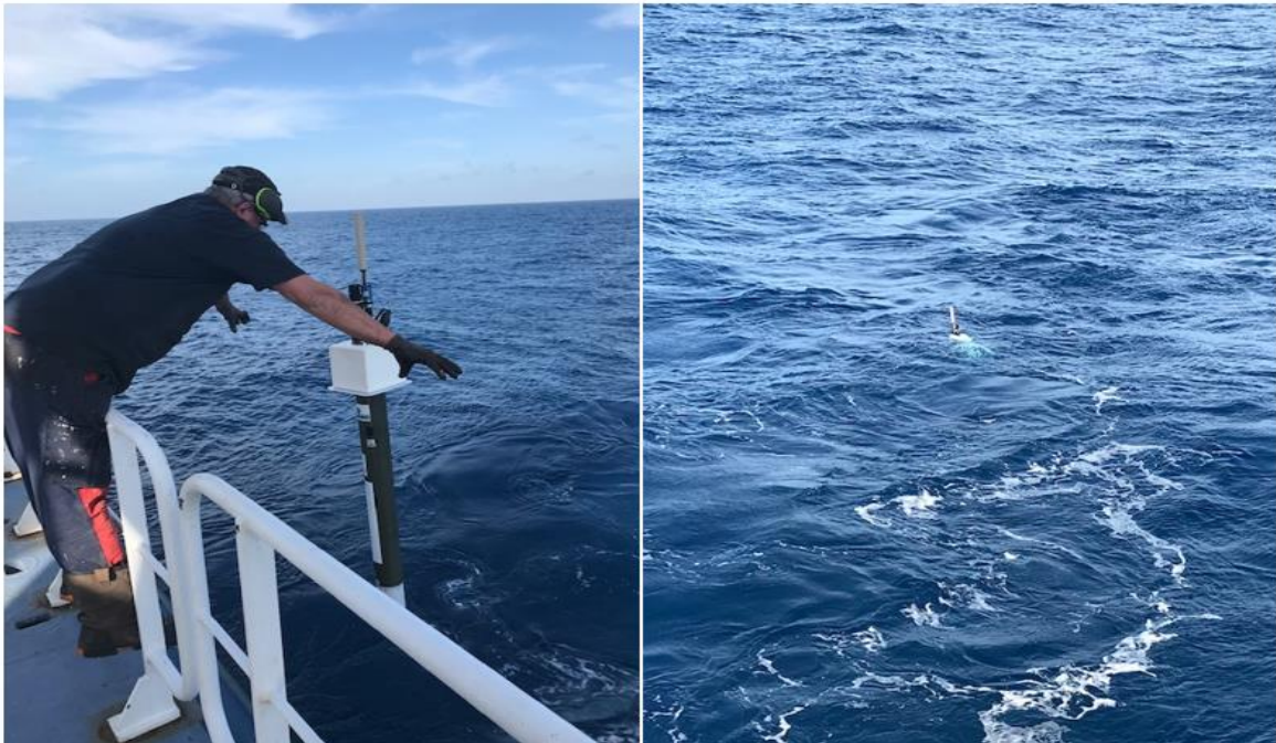
Figure 1. Arvor-I deployment from R/V Pourquoi Pas? in the eastern Mediterranean in March 2019.
