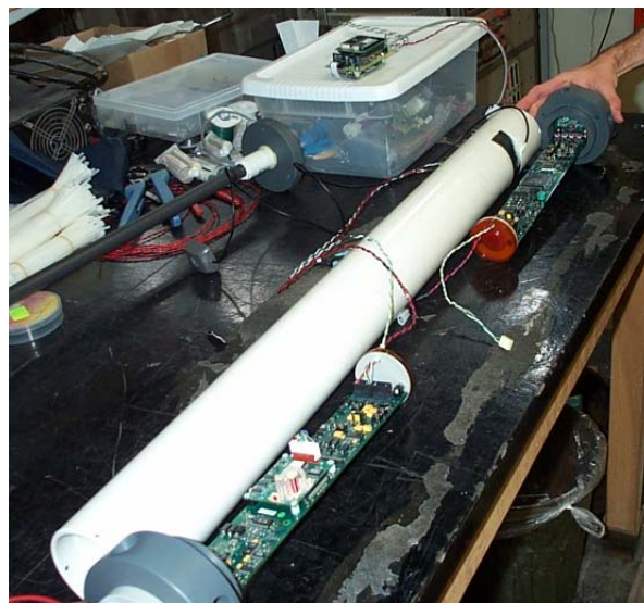
Figure 2. Photograph showing how the two Nortek Aquadopp currentmeters were fitted inside the tubular body of the CODE drifter.
