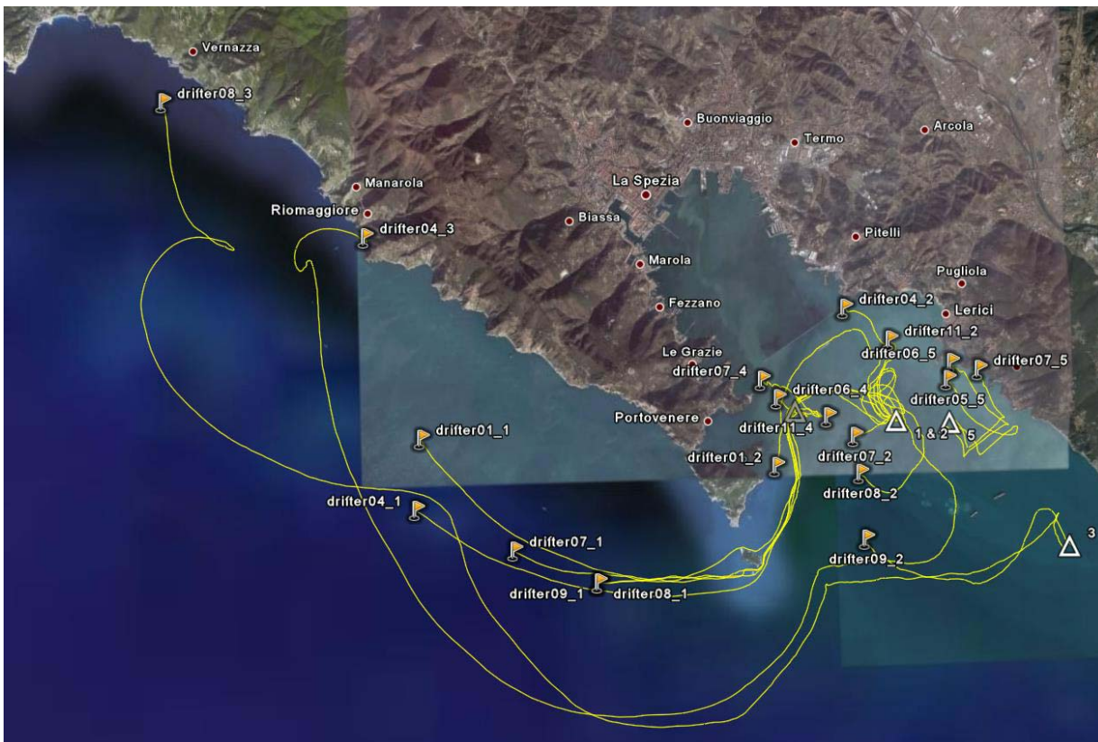
Figure 34. Composite plot with edited trajectories of drifters released during all the dispersion experiments in the vicinity of the GSP (18-26 June 2007).
