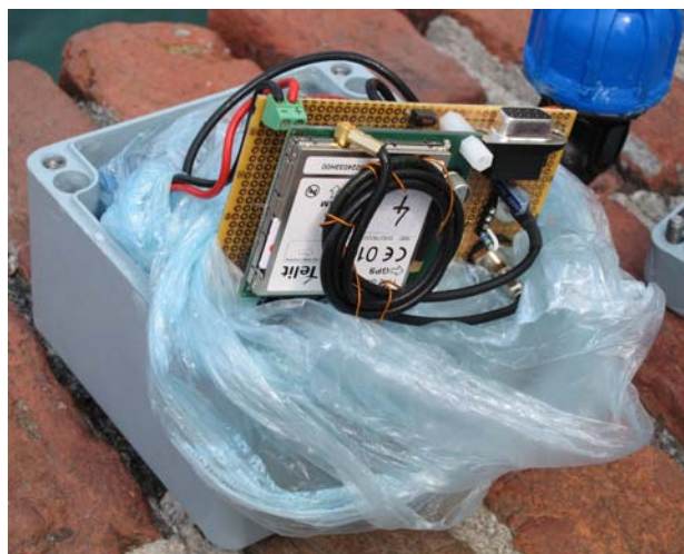
Figure 1. Telit GPS and GSM/GPRS module, electronic circuit, and batteries (in plastic bag) included in the waterproof container.
