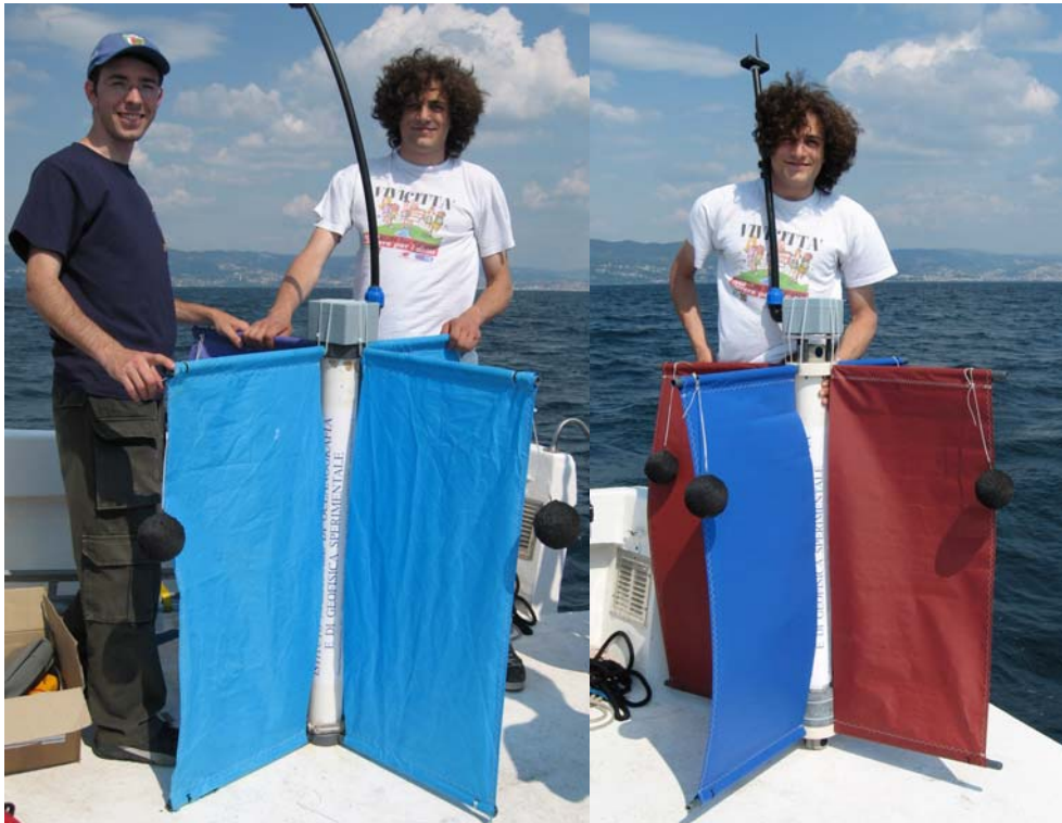
Figure 3. Pictures of CODE drifters equipped with GSM/GPS electronics (in cubic container) and dual antenna: regular drifter (left) and drifter fitted with Nortek Aquadopp currentmeters (right).
