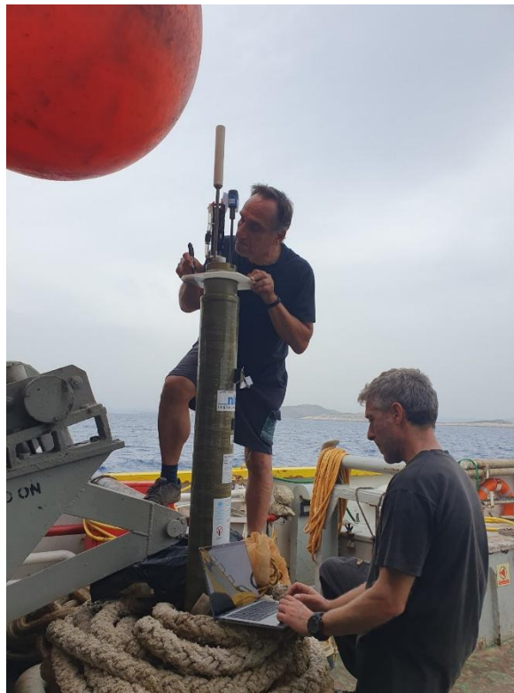
Figure 6. Arvor-D DO WMO 3902483 in the Ionian Sea from M/Y AEGAEO (credit HCMR).
